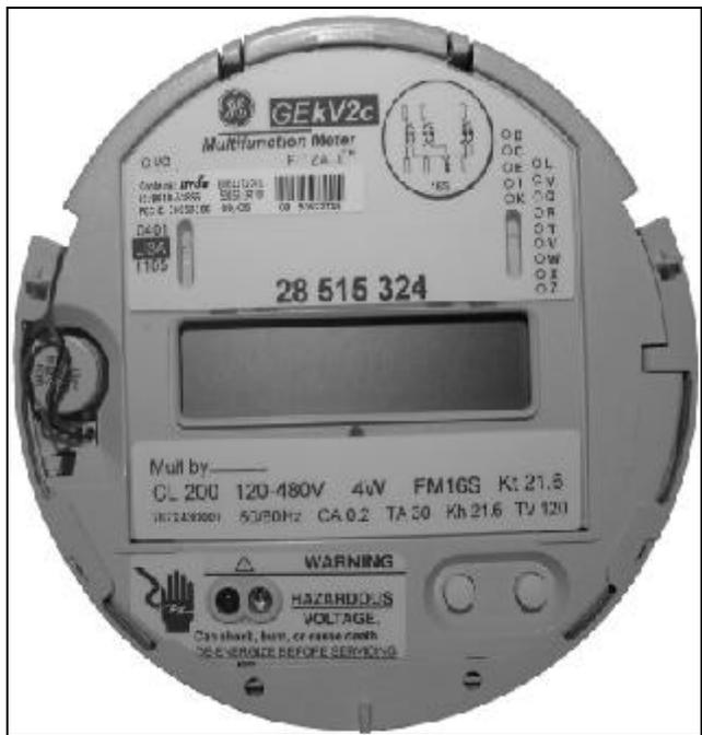
KV2c retrofitted with 53ESS Itron module/
