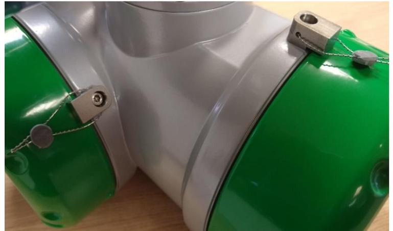
**Figure 3.** Sealing of the caps on the CFT34A |
