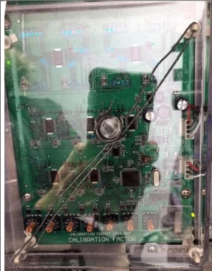
Figure 6 Sealing the Metrological circuit board |
