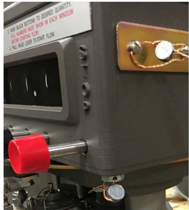
Fig. 2 – sealing points/ points de scellage
