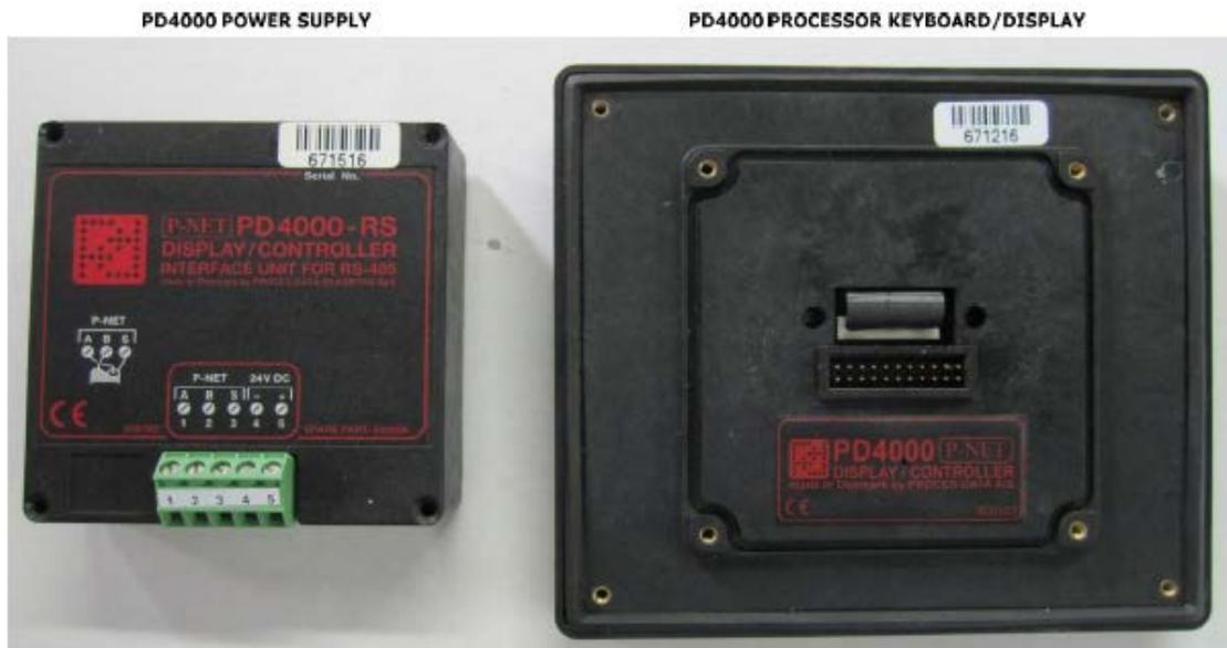
**Fig. 2 :** Power supply unit taken apart from the PD4000 UPI controller to access the W&M Lock
