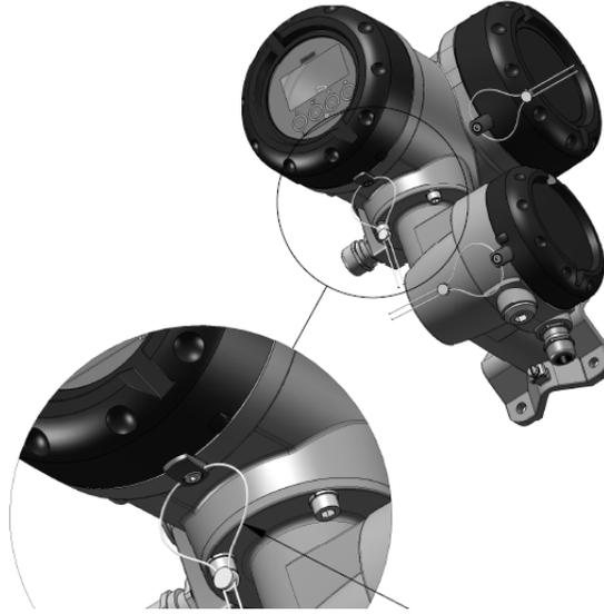
Figure 2: Sealing of the three caps on the LCI 40
