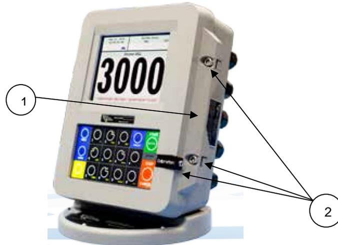
**Figure. 4:** TCS 3000 Register Sealing and Marking Locations/
