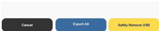
Selecting “Export All” will transfer all Batch and Transaction log files including the “Audit Trail Log” and the “Event Log” files onto the USB memory stick so that they may be viewed using a normal text editor from a lap top computer.
