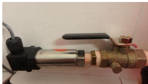
Figure 4: Level sensor and simulation valve | Sonde de niveau et soupape de simulation
