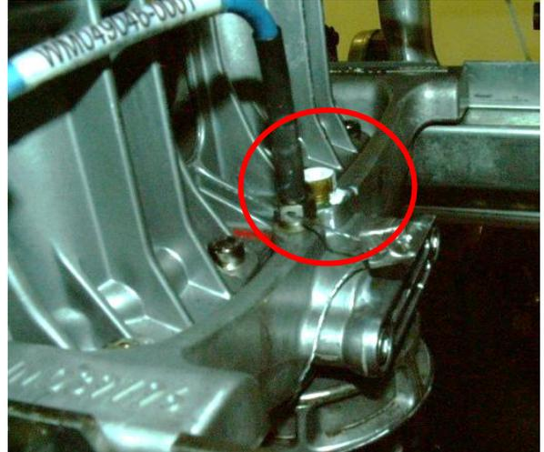
Figure 12: Side of Xflo meter with the ATC temperature probe and thermowell /
