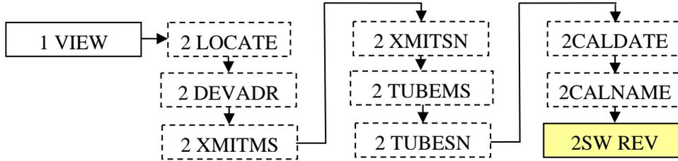
Chart 3. “View” menu to view software version (2SW REV) on local display of CFT51 (Figure 1). *Note: Modbus view shown here; For HART, scroll down until reaching 2SW REV in the same manner.*
