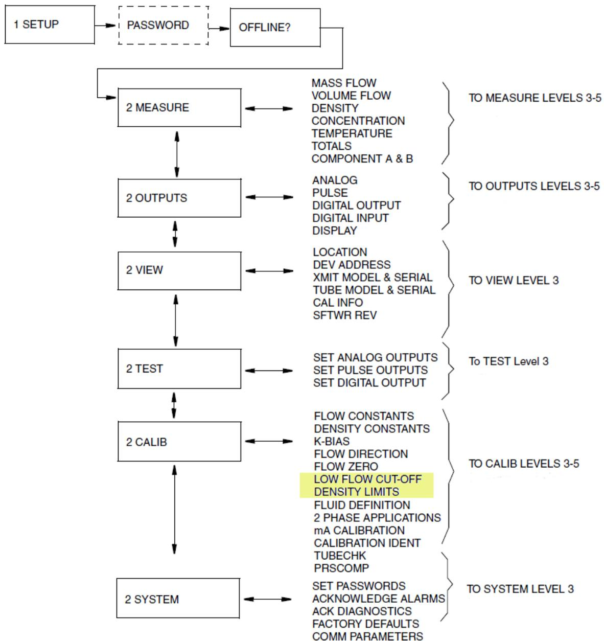
Chart 2. SETUP Menu Structure; Low Flow Cut-Off and Density Limits parameters can be viewed and set through the above sequence. *Note: The "2 MEASURE" should be accessed through level 1 (1 SETUP) by entering the setup mode, not by scrolling down to "1 MEASURE".*
