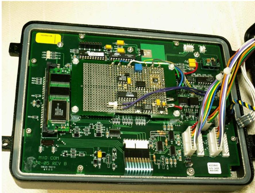
As a result of a change in the type of temperature probes used with the E:Count register, additional electronic components were added to the original circuit board. These include a piggy back board with jumper wires connected to the appropriate points, as seen in the diagram above.
