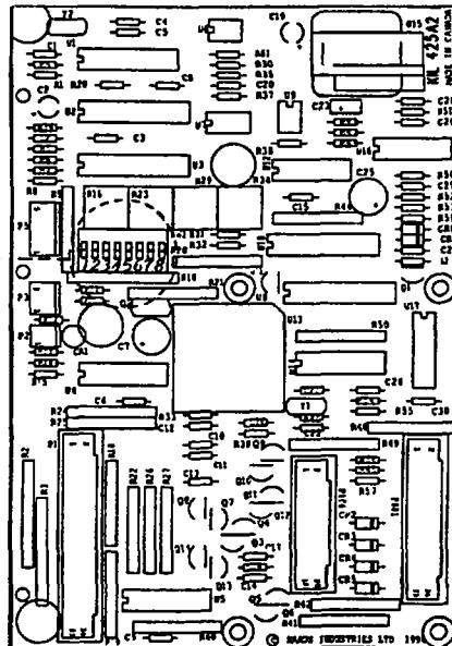
The temperature, flow and volume board is used to display the gross volume, flowrate and temperature of the product desired. To view this information, the three switches are set in accordance with Figure 2 as indicated. When the GTC 200 is installed inside the model ECW Salesmaker Pro-Blender, the blend ratio is displayed at any time during a delivery by setting switches SW2 and SW3 in the up position.
