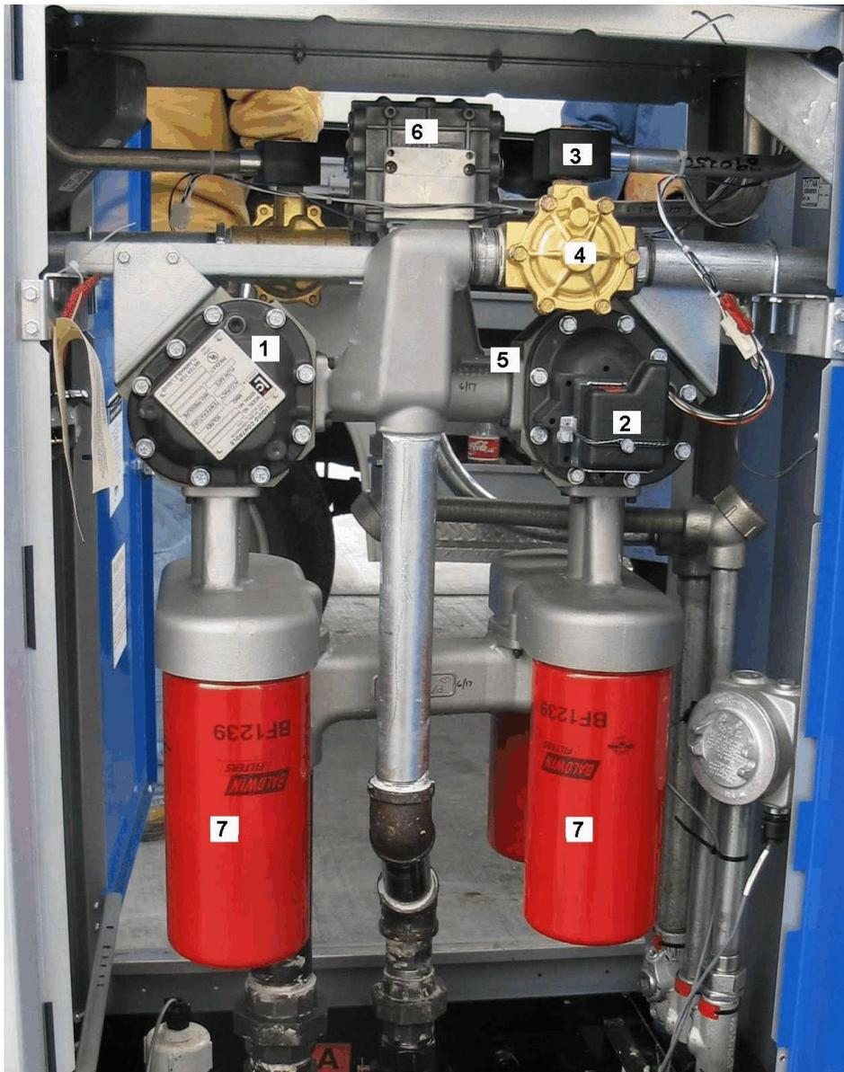
**Fig. 7: Hydraulic structure of UHC dispensers |
