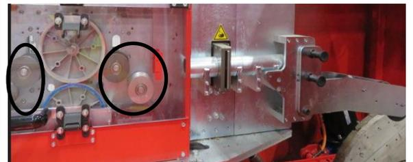
**Typical centering mechanism with adjustable V-rollers (circled) on both
