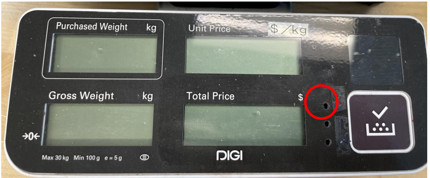
SBS-1000 Recessed SAZM button circled in red / Touche SAZM encastré encadré en rouge SBS-1000
