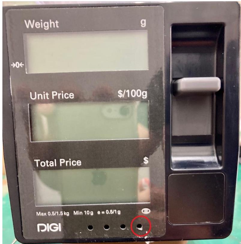
HS-1000 Recessed SAZM button circled in red / Touche SAZM encastré encerclé en rouge HS-1000
