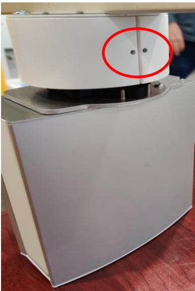
Typical sealing for collar bracket (housing)/
