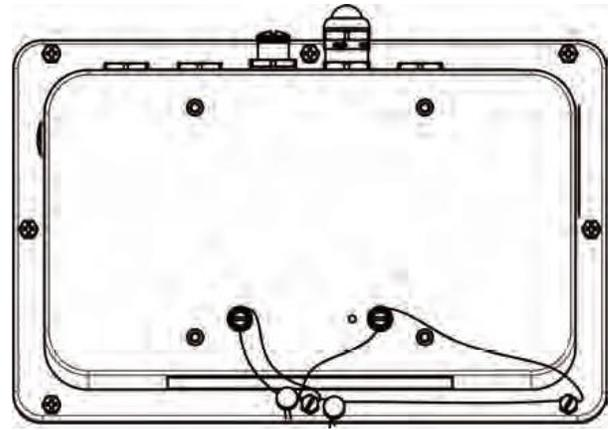
Wire seal with two load receiving éléments /
