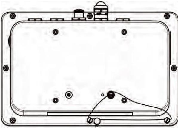
Wire seal with one load receiving element /
