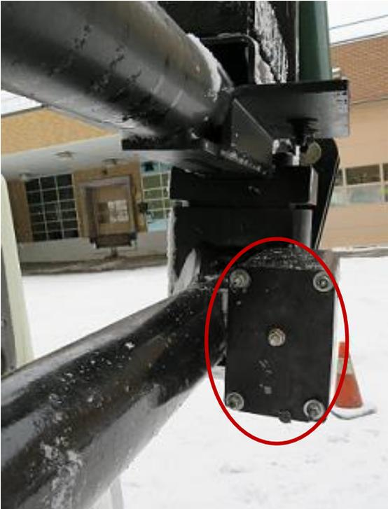
**Typical sealing for the fork angle sensor and amplifier /
