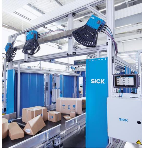
Typical Dimensioning Arrangement VMS5300 /
