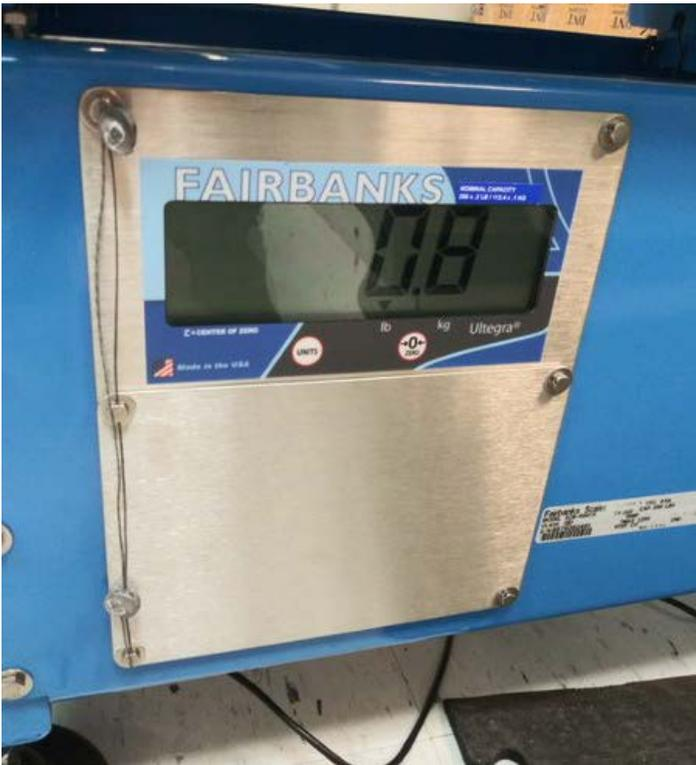
**Typical Sealing / Scellage typique**
