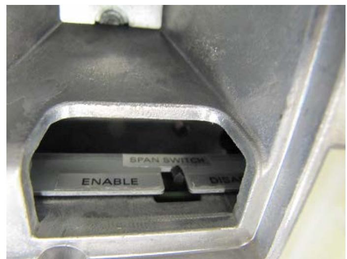
Typical calibration switch access /
