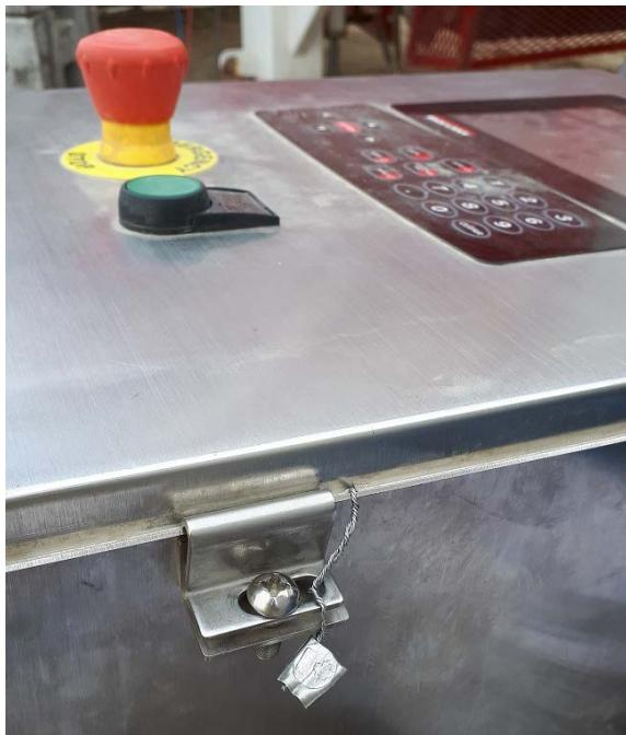
**Sealing of indicator, to prevent access to inclinometer and cleanout time push buttons /**
