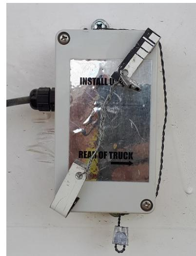
**Sealing of the inclinometer, one seal to secure the box to the frame and another to prevent access to the box /**
