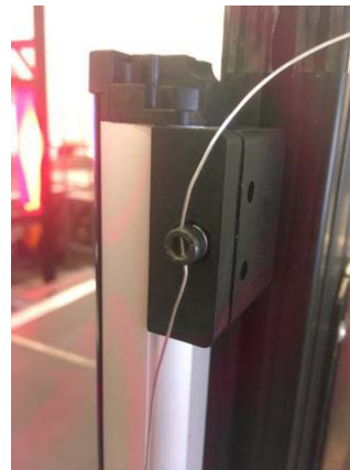
Typical sensor head sealing (only 1 screw shown) / Scellage typique des capteurs (une seule vis est visible)
