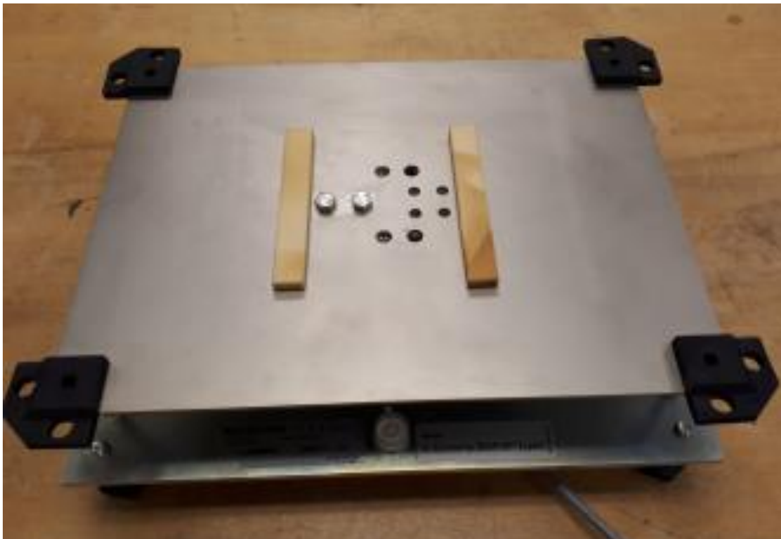
Typical SP4M C6 MR 15 kg, PC 6 C3 20 kg Y=12500 and SP4M C3 MR 30 kg Sub-platter / Sous-plateau SP4M C6 MR 15 kg, PC 6 C3 20 kg Y=12500 et SP4M C3 MR 30 kg typique
