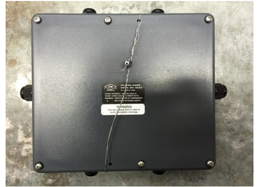
Typical Sealing / Scellage typique
