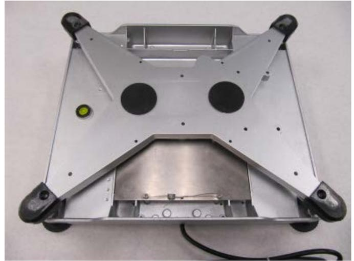
**Typical sub-platter and sealing / Sous-plateauet scellage typique****PARTIE 9 - Évalué par**
