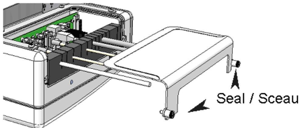
Typical sealing of connector cover plate / Scellage typique du couvercle du panneau de raccordement
