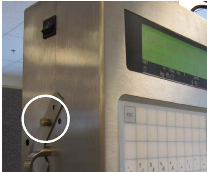
**Typical sealing location / Emplacement typique du sceau physique (UNI-3 L2H)**
