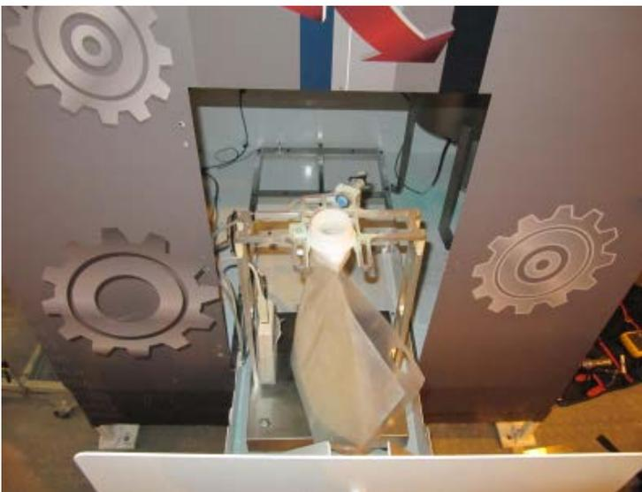
**Typical load receiving element with bag mounted / Dispositif
