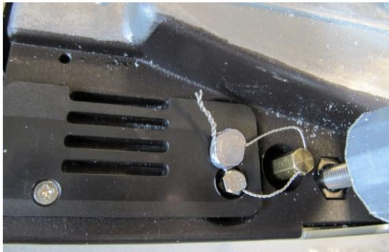
**Typical seal method for housing access/
