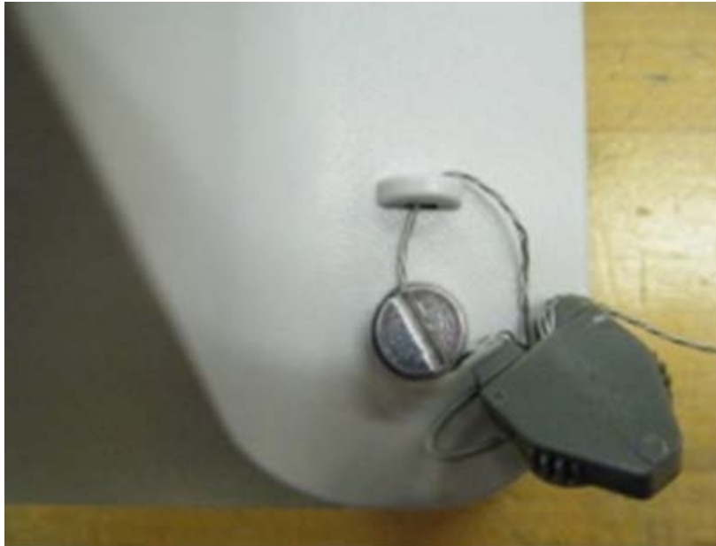
Typical sealing of model IND231 / Scellage typique du modèle IND231
