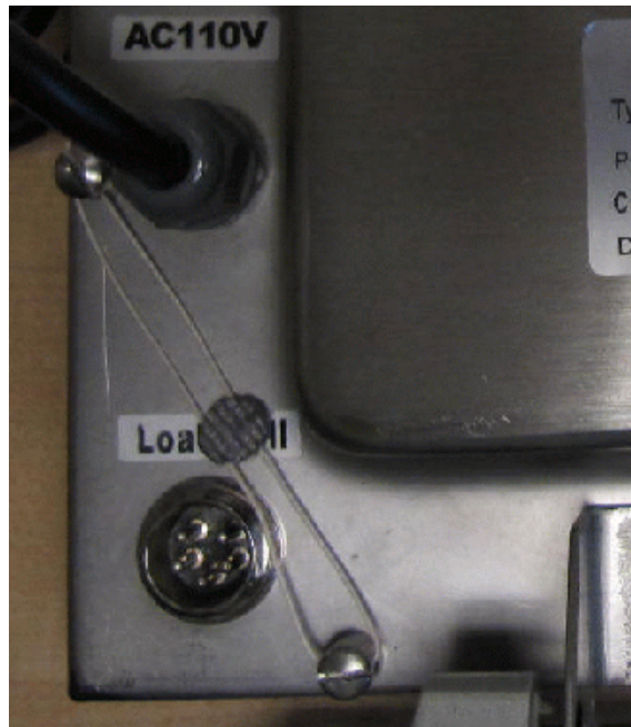
Typical sealing / Scellage typique
