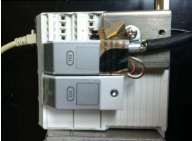
Typical sealing of model WM-3 Weighing Module / Scellage typique du modèle WM-3 Weighing Module
