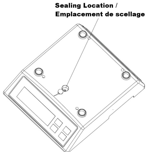
**Typical sealing method / Methode de scellage typique**
