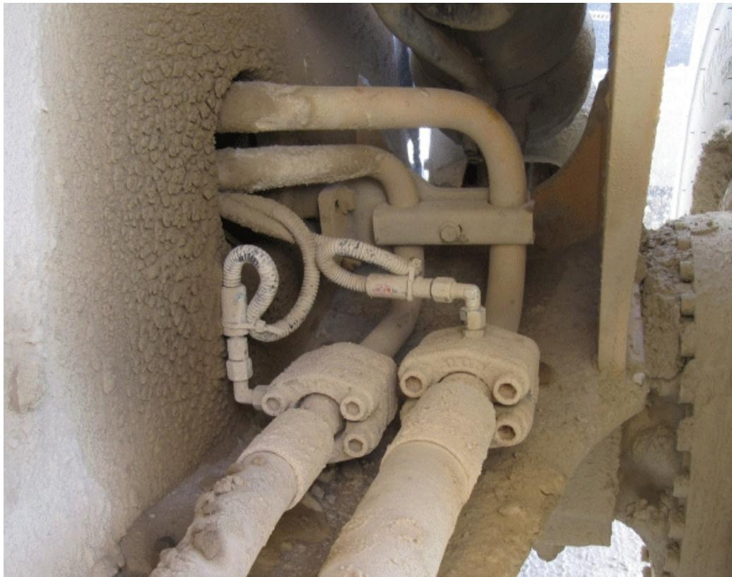
**Typical pressure transducer installation /
