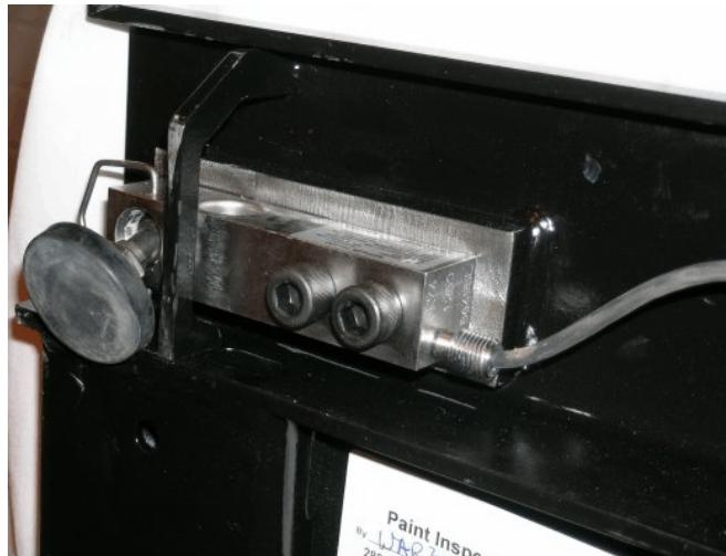
Typical load cell installation
