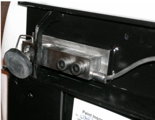
**Typical load cell installation
