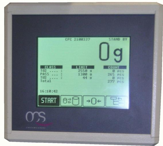
**Typical model RC-TERM operator display/
