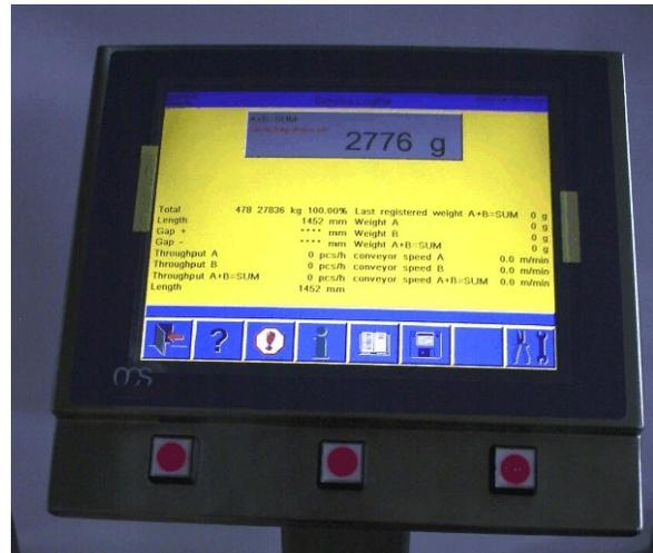
**Typical pole mounted HC Bedienterminal operator
