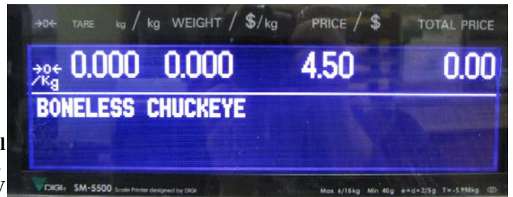
Typical customers' display for SM-5500 Audit Trail series models / Affichage destiné aux clients typique des modèles du series SM-5500 Audit Trail
