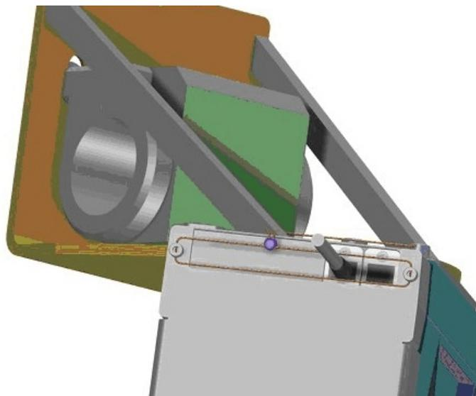
**Typical Sensor Head Connector Hood Sealing / Scellage typique du
