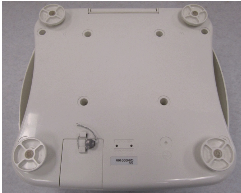
Typical sealing / Scellage typique
