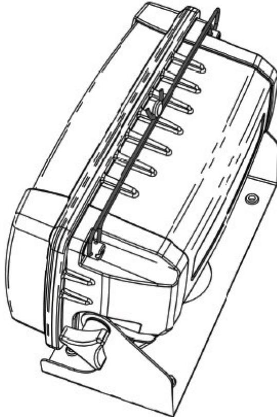
**Typical model 250X sealing method/
