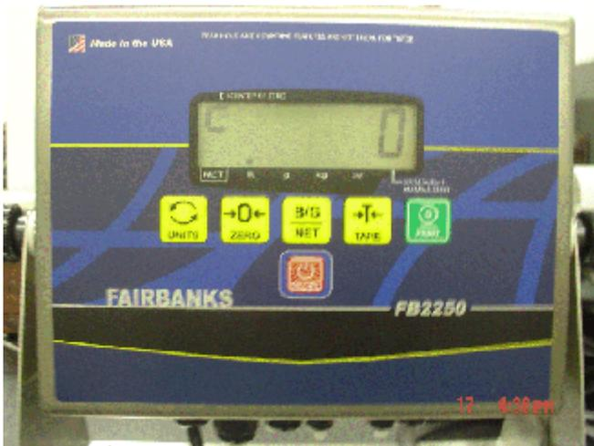
**Typical FB2250-X indicator with stainless steel housing /
