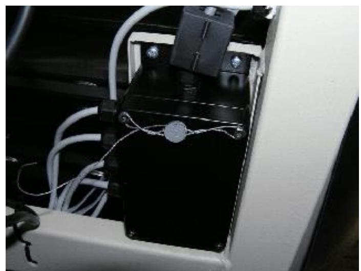
Typical sealing of Junction box with wire seal /
