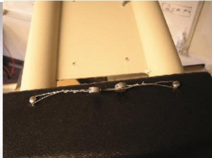
Sealing of Height Sensor for CubiScan 150-LFT /
