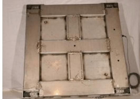
**Bracing Structure / structure de renforcement**
