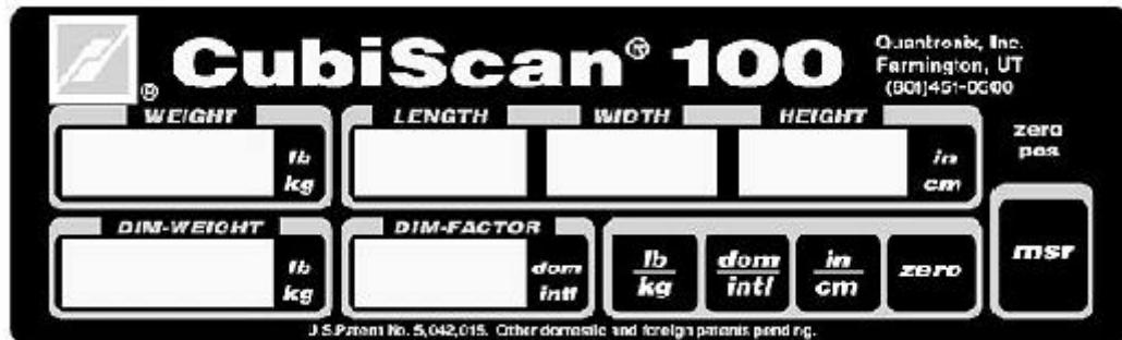
All controls and displays are located on the control panel at the front of the base.
