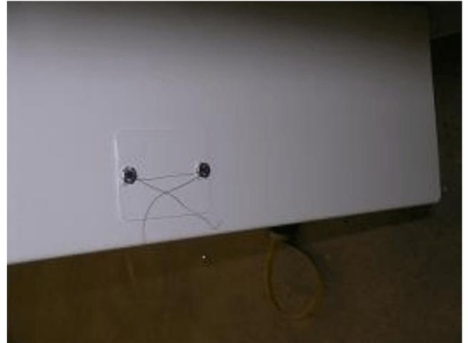
Typical sealing means / Dispositif de scellage type
