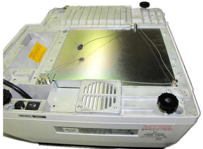
Typical sealing of models SM-100***BCS, SM-100***BCS+, SM-100***PCS and SM-100***PCS+ / Scellage typique des modèles SM-100***BCS, SM-100***BCS+, SM-100***PCS et SM-100***PCS+
