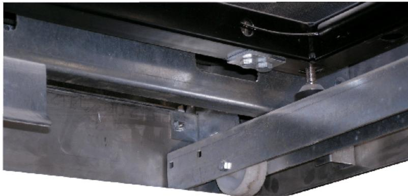
**Typical support frame showing wheel mounting and adjustable feet locations / Châssis de support
