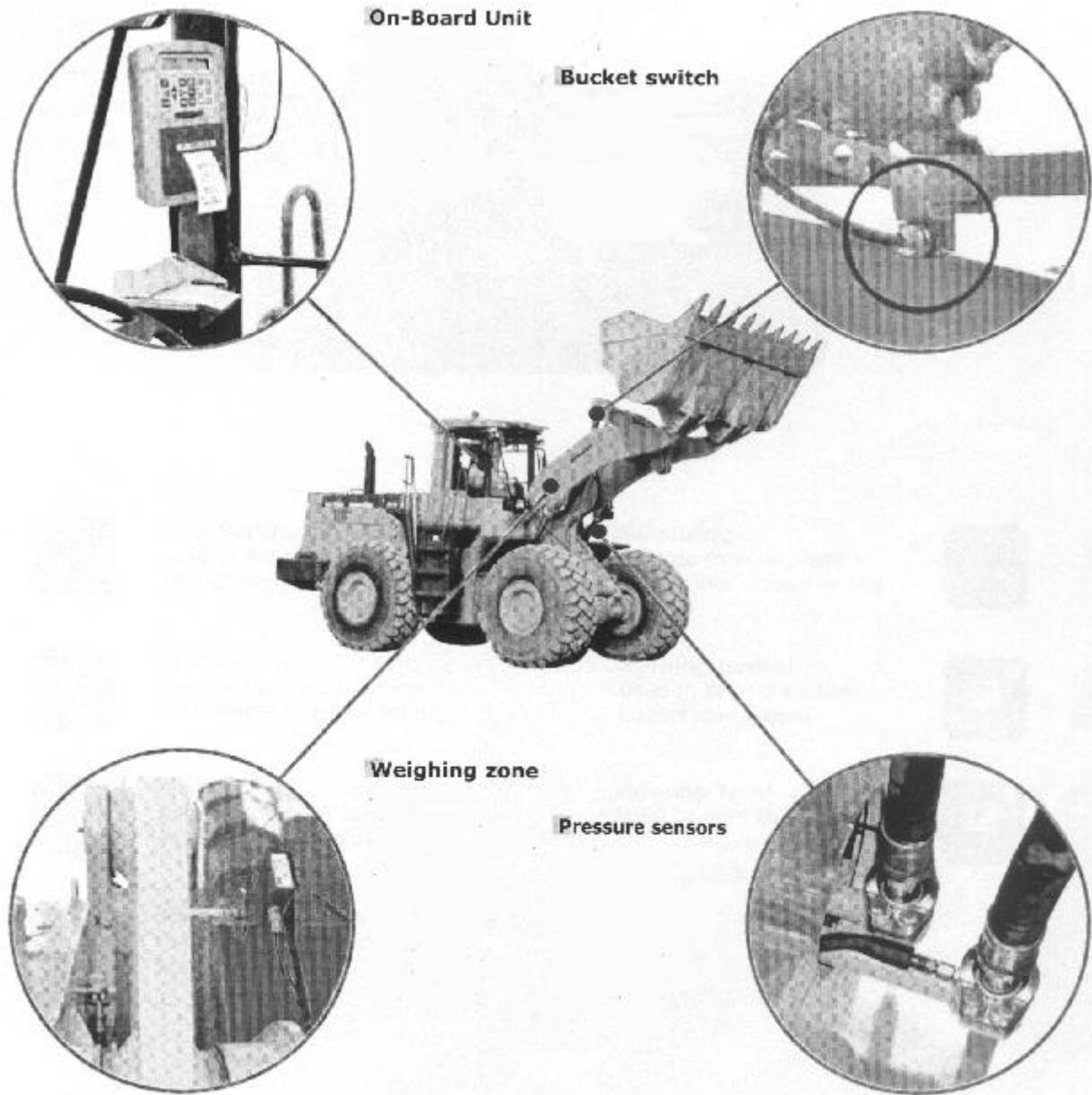
**Typical Components Installation on the Dozer Loader Weighing System /**
